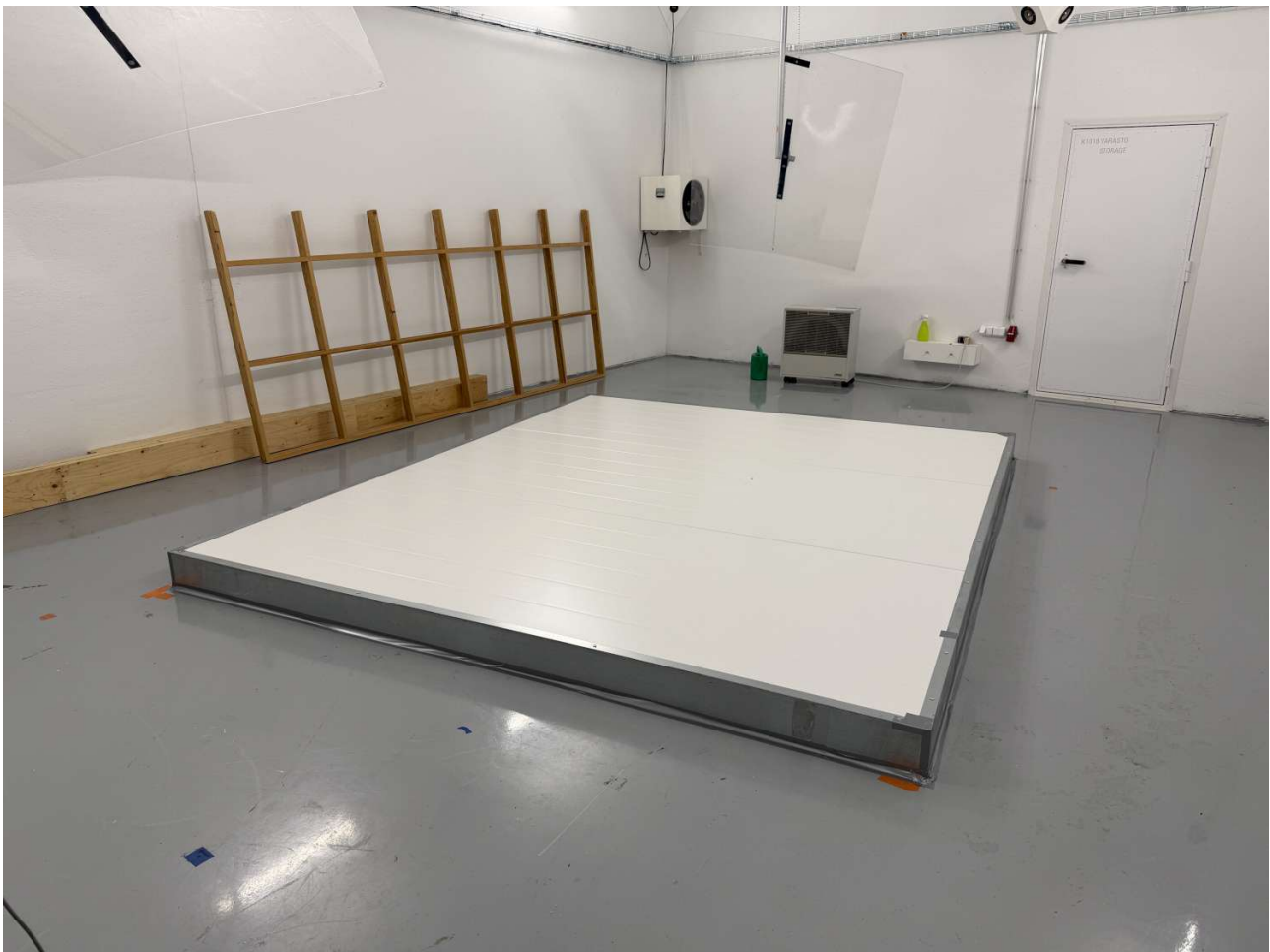
Figure A3.1. The specimen mounted on the floor of the reverberation room perforated side against the floor.
