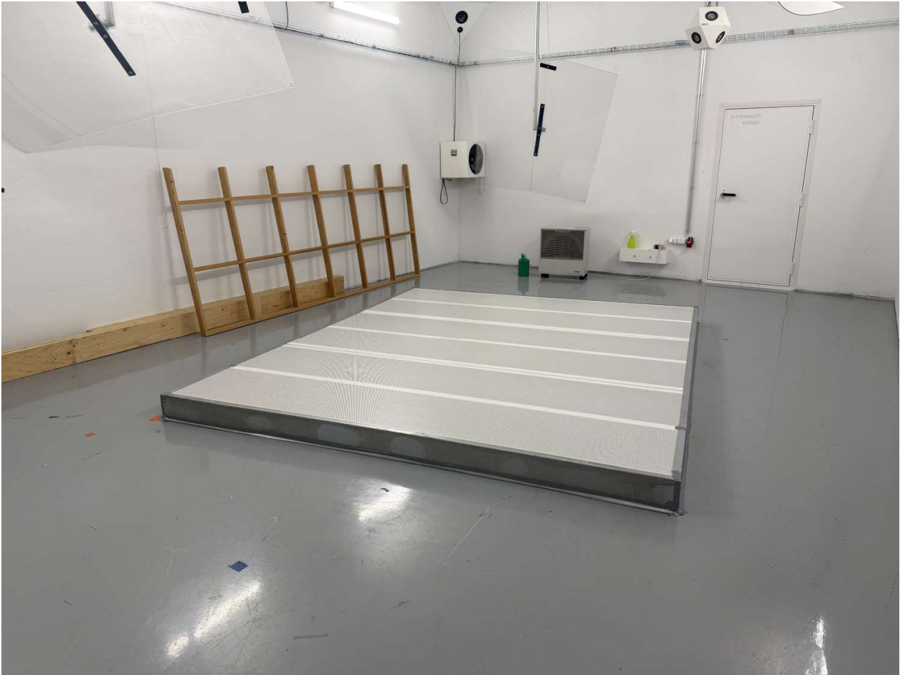
Figure A3.2. The specimen mounted on the floor of the reverberation room perforated side up.
